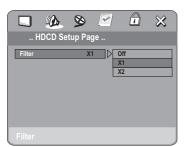
**OFF**: HDCDs will be played like normal audio CDs. **1X (44.1K) or 2X (88.2K)**: HDCDs will be played at a sampling frekquency of 44.1KHz or 88.2KHz if possible. (This setting depends on the contents of the disc).
